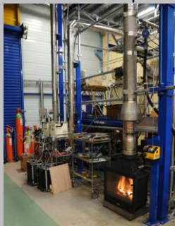
INERIS dilution system for Wood stove / Fireplaces
